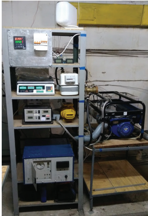
Fig. 1. General view of experimental bench based on the engine with spark ignition 1Ch 6.8/5.4
