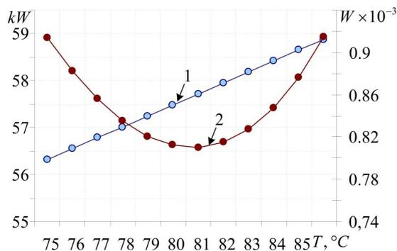
Fig. 11. Change of energy consumption and wear of heaters depending on the change of the reference value of the temperature parameter of the second module in the three-modular heating system: 1 – energy consumption value; 2 – wear value of electric heaters
