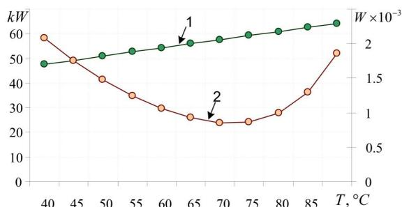
Fig. 7. Change of energy consumption (1) and wear of heaters (2) depending on the change of the temperature parameter reference value of the first module in the two-modular heating system
