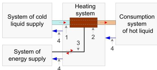
Fig. 3. The structural diagram of interaction of one heater heating system with the counterpart systems: 1 – end-to-end channel of liquid movement; 2 – technological heating mechanism; 3 – energy supply channel; 4 – control channels
