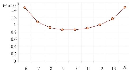
Fig. 9. Dependence of the heater wear value on the number of heating sections which are parts of the first module
