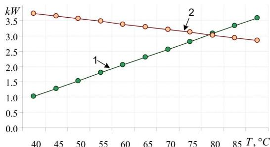
Fig. 6. Changes of the given electric power on heating modules sections depending on the established first module temperature reference value: 1 – change of energy supply on the first module; 2 – change of energy supply on the second module
