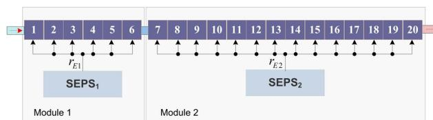
Fig. 8. The principle of redistribution of heating sections between modules
