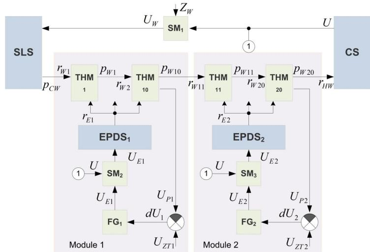
Fig. 4. Structural diagram of the dynamic fluid heating system with two sectional stabilization modules: SLS – cold liquid supply system; CS – system of heated liquid consumption; EPDS – energy product delivery system; THM – technological heating mechanism; SM – synchronization mechanism for data transmission; FG – functional generator
