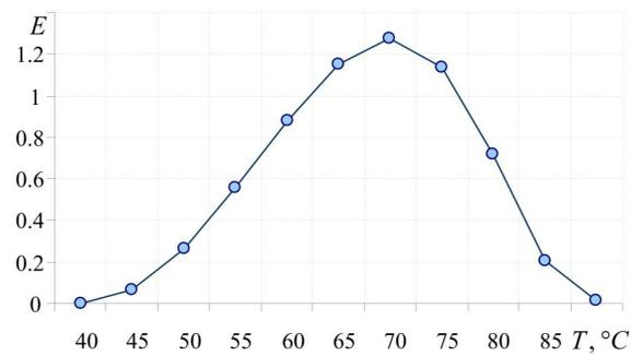
Fig. 12. Changing the resource efficiency in the two-module heating system with the temperature parameter change of the first module
