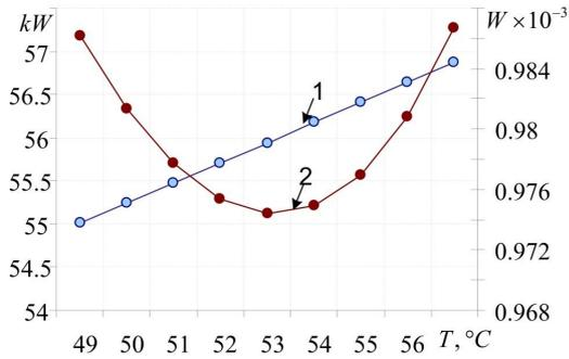
Fig. 10. Change of energy consumption and wear of heaters depending on the change of the temperature parameter reference value of the first module in the three-modular heating system: 1 – energy consumption value; 2 – wear value of electric heaters
