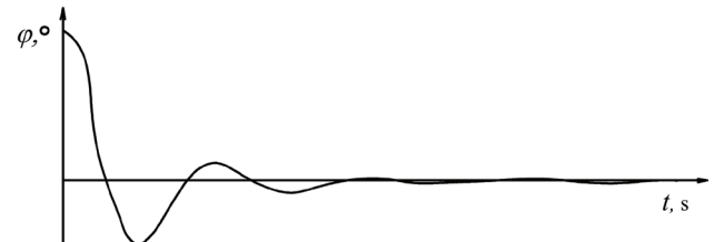
Fig. 5. Character of damping the perturbed motion of a direct seeding seeder
