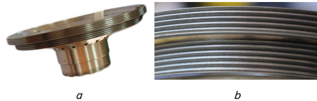
Fig. 1. Covering disk of the GTE turbine, the TV3-117 family: general view (a); the labyrinth seal ridges (b)
