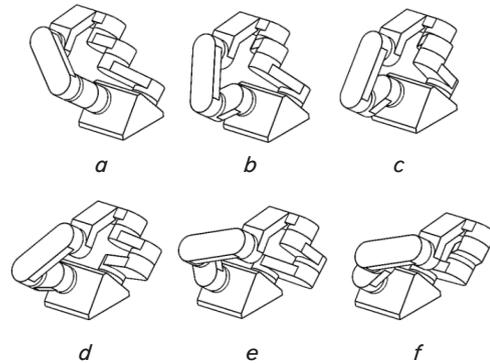
Fig. 7. The positions of the links of an arbitrary SHSLLM: a–f are the successive positions of the links through the same intervals of movement of the final link within the working range
