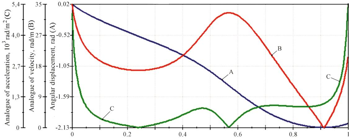
Fig. 8. Kinematic diagrams of a long lever of a reciprocal coupled SHSLLM of unilateral joining (A – angular displacement, B – analogue of velocities, C – analogue of accelerations by the module)
