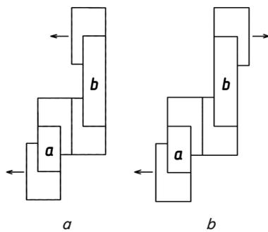
Fig. 10. Compounding types of pairs of levers: *a* – one-way connection; *b* – two-way connection
