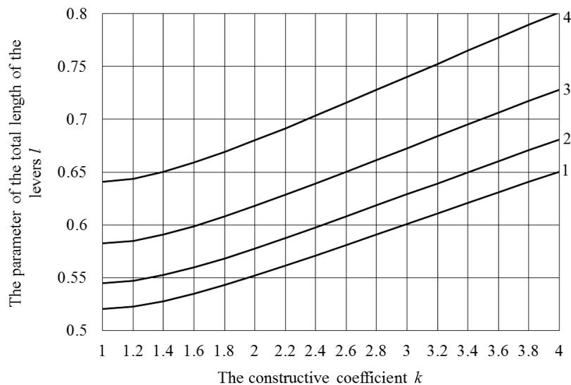
Fig. 5. The nomogram of the influence of the constructive coefficient  $k$  on the parameter  $l$  of a pair of levers
