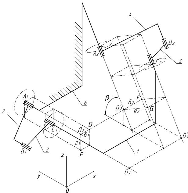
Fig. 2. A scheme of the SHSLLM with arbitrary dimensions, interaxial distances and displacements
