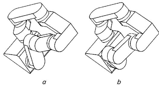
Fig. 11. Variants of the SHSLLM with different arrangements of levers in a pair of two-way joining: *a* – initial; *b* – changed; 1 – a short lever; 2 – a long lever
