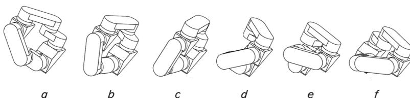
Fig. 14. A symmetrical SHSLLM: *a–f* are the successive positions of the links of the mechanism through identical intervals of movement of the final link within the working range
