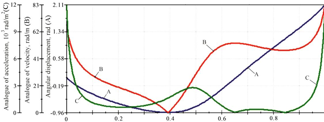
Fig. 9. Kinematic diagrams of a short lever of a reciprocal coupled SHSLLM of unilateral joining (A – angular displacement, B – analogue of velocities, C – analogue of accelerations by the module)
