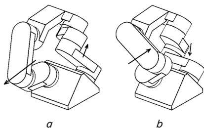
Fig. 12. Variants of the SHSLLM with different characteristic positions of both pairs of levers: *a* – initial; *b* – changed
