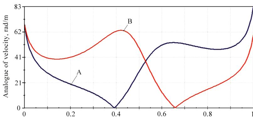
Fig. 13. Distribution of maximum velocities and points of stops of short levers (curves A and B) of opposite lever pairs in the coordinates of the movement of the final link
