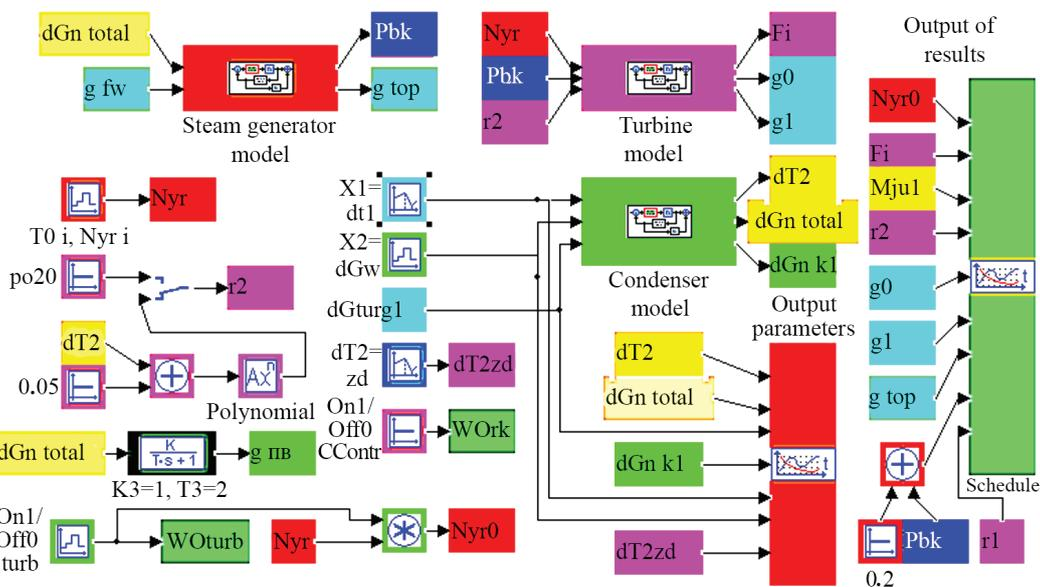
Fig. 2. Block diagram of algorithms for the calculation of dynamic processes of interaction of automatic controllers in the MEC control system
