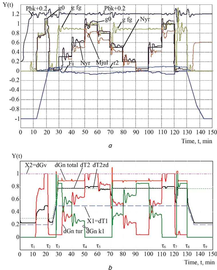
Fig. 4. Graphs of transients: *a* – in the turbine and steam generator; *b* – in the condenser, in the interaction of all controllers and step variation of the turbine load
