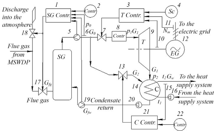
Fig. 1. Block diagram of the MEC-5 control system
