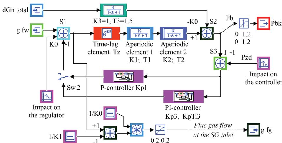
Fig. 3. Block diagram of algorithms for the calculation of dynamic control processes of the SG outlet steam pressure
