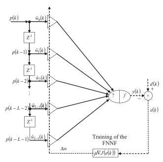
Fig. 11. Focused neural network filter based on a linear adaptive adder
