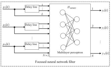
Fig. 12. Embodiment of SNF for the MIMO transmission system
