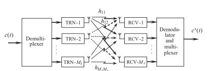
Fig. 1. Block diagram of the MIMO system
