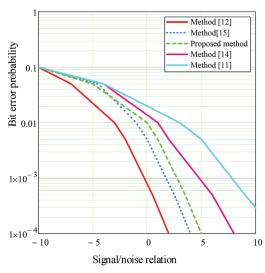
Fig. 10. Dependences of the bit error on the signal/interference ratio for the developed integrated estimation method and the methods considered in studies [11, 12, 14, 15]
