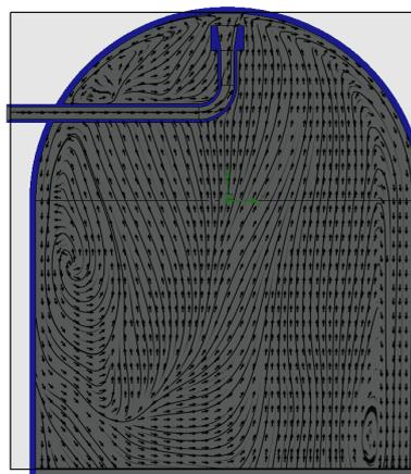
Fig. 3. Trajectories of gas motion inside the body of the damping attachment
