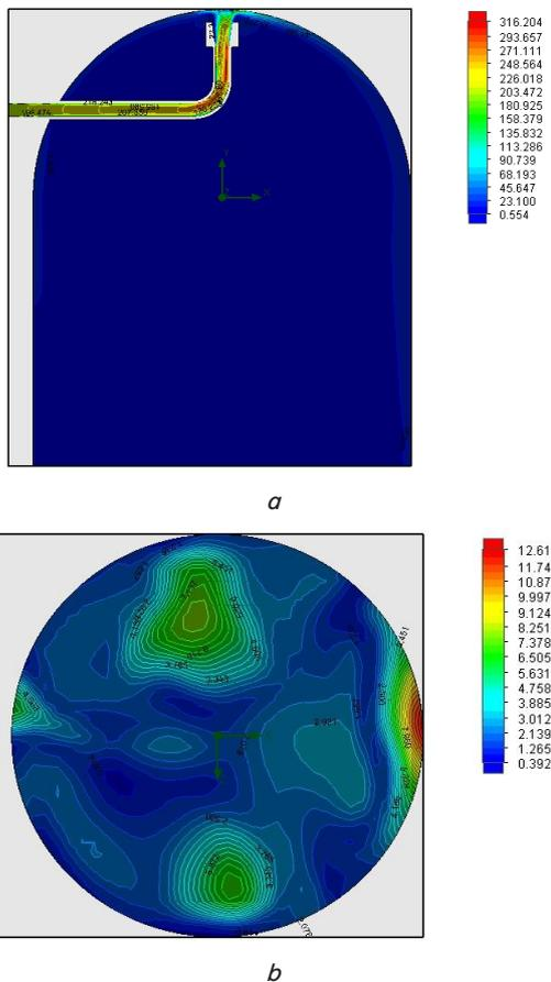
Fig. 2. Chromogram of gas leakage: *a* – vertical symmetrical cross-section; *b* – horizontal cross-section at the outlet
