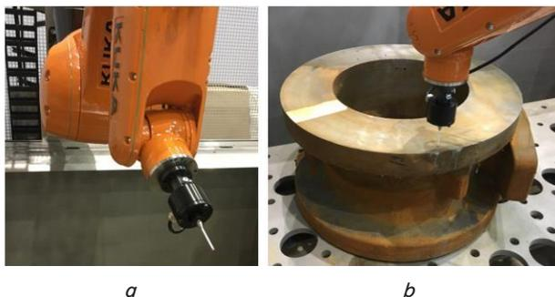
Fig. 5. Obtaining data with the contact measuring tool:
