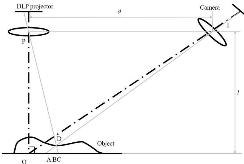
Fig. 1. Structured light scanning principle
