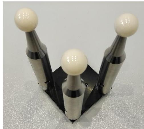
Fig. 3. Reference sample for calibration of the visual testing system
