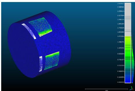
Fig. 9. Distribution of the distances from each point to the 3D model
