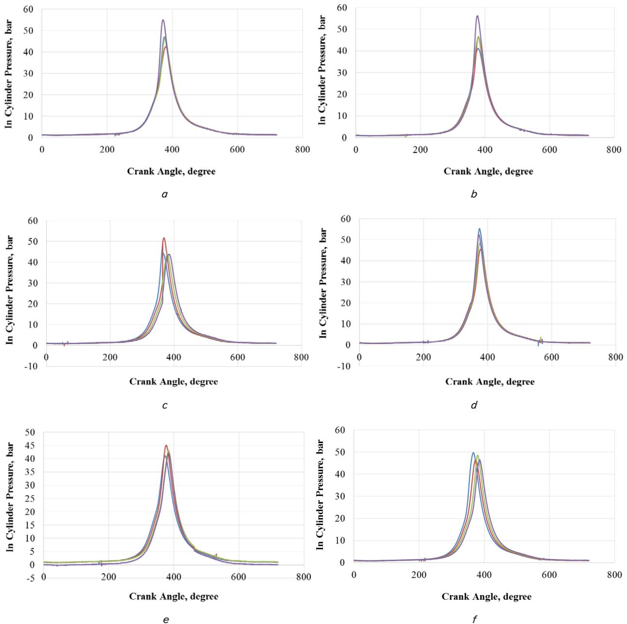
Fig. 2. In-Cylinder Pressure VS Crank Angle on Fuel Mixture Variations at 6,000 rpm:
