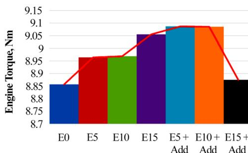
Fig. 6. Maximum Torques of 7 Fuel Variations
