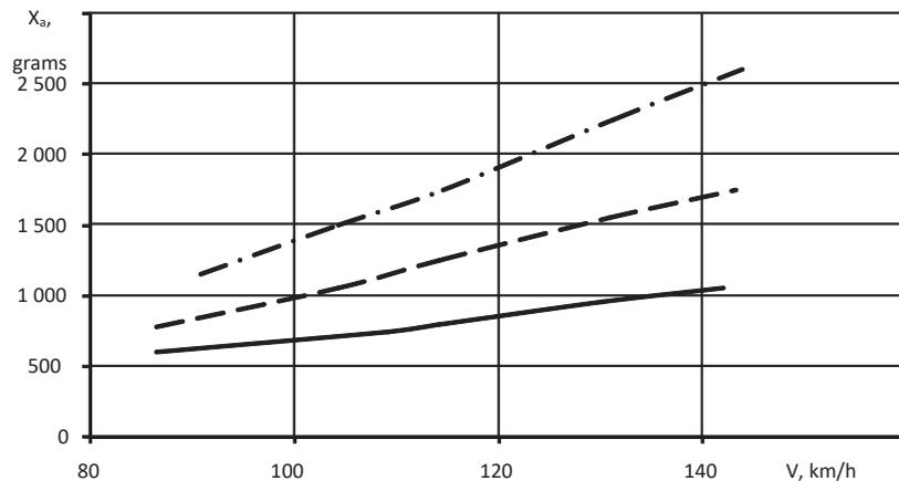
Fig. 4. Dependence of the model’s frontal drag on speed in ADC working section; the model is near the screen’s surface (— – model with a passage; - - - - - model with a closed external contour; - · - - - model with a fully closed input)
