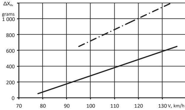
Fig. 5. Dependence of an increase in the model's frontal drag on speed in ADC working section; no influence from the underlying surface (— — model with a closed external contour; - · - - model with a fully closed input)
