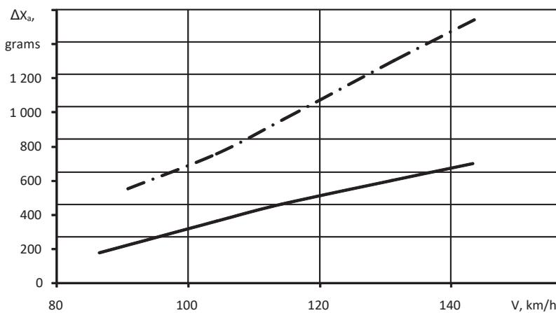
Fig. 6. Dependence of an increase in the model's frontal drag on speed in ADC working section; the model is near the screen's surface (— — model with a closed external contour; - · - - model with a fully closed input)
