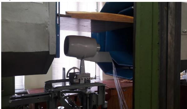
Fig. 1. Photograph of the physical appearance of a working part of the wind tunnel T-1 with a model of the two-circuit engine
