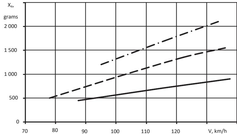
Fig. 3. Dependence of the model’s frontal drag on speed in ADC working section; no influence from the underlying surface (— – model with a passage; - - - - - model with a closed external contour; - · - - - model with a fully closed input)
