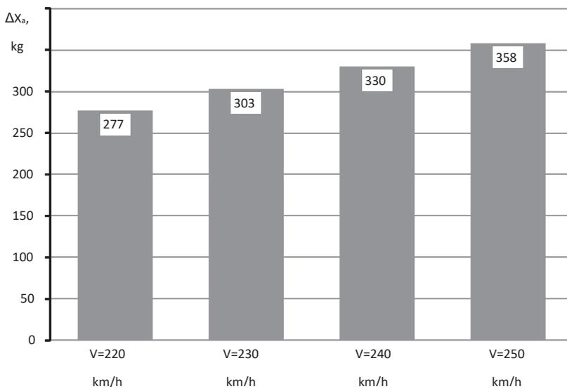
Fig. 7. Magnitudes of increase in TJTE nacelle's frontal drag at a fully closed input to the engine with a by-pass ratio  $m=20$  and different aircraft landing speeds
