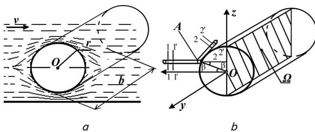
Fig. 2. General view of a stone: *a* – in a flow; *b* – interaction between an arbitrary elementary jet and a cylindrical stone
