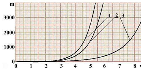
Fig. 5. Dependence of mass  $m$  (kg) of individual stones that shift after a river flow reaches velocity  $v$  (m/s): 1 – for  $Y_s=0.9$ ; 2 – for  $Y_s=1.0$ ; 3 – for  $Y_s=1.5$
