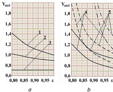
Fig. 4. Dependence of streamlining coefficient  $Y_{strl}$  on a flow compression coefficient  $\epsilon$ :  $a$  – 1 – spherical and ellipsoidal, 2 – cylinder, 3 – parallelepipedal stones;  $b$  – 4 – pyramidal, and 5 – wedge-shaped stones; for diagrams 4 and 5: solid lines correspond to  $\theta=45^\circ$ , dashed lines –  $\theta=40^\circ$ , stroke-dotted lines –  $\theta=30^\circ$
