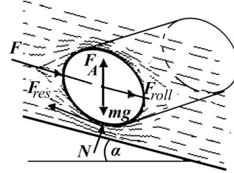
Fig. 3. The limit of a stone equilibrium in a descending flow of fluid:  $F_A$  – pushing force,  $F_{res} = (\rho_s - \rho_w) V_T g f \cos \alpha$  is the resistance force,  $F_{roll}$ ,  $N$  is the rolling force and the normal reaction from a bottom
