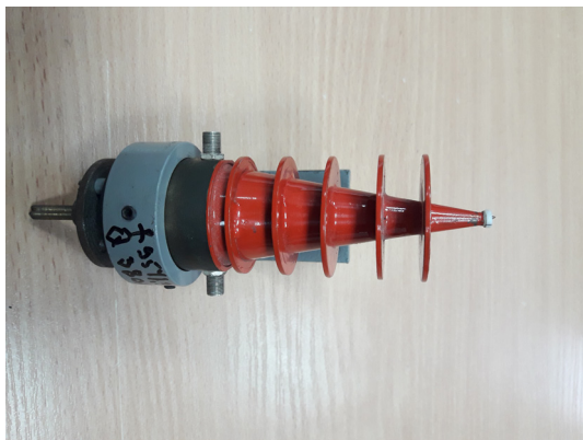
Fig. 9. Physical appearance of the experimental prototype of RMT based on an irregular coaxial structure
