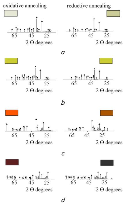
**Fig. 2.** Bar radiographs of ceramic clinker samples of different color, annealed in the oxidative and reductive environment: *a* – creamy; *b* – yellow; *c* – red; *d* – brown. ▲ – quartz; ● – albite; △ – microcline; ▴ – hedenbergite; ■ – mullite; ▮ – rutile; ○ – hematite; ⊙ – magnetite; ◻ – gaussmanite; ⊠ – Mn<sub>2</sub>O<sub>3</sub>
