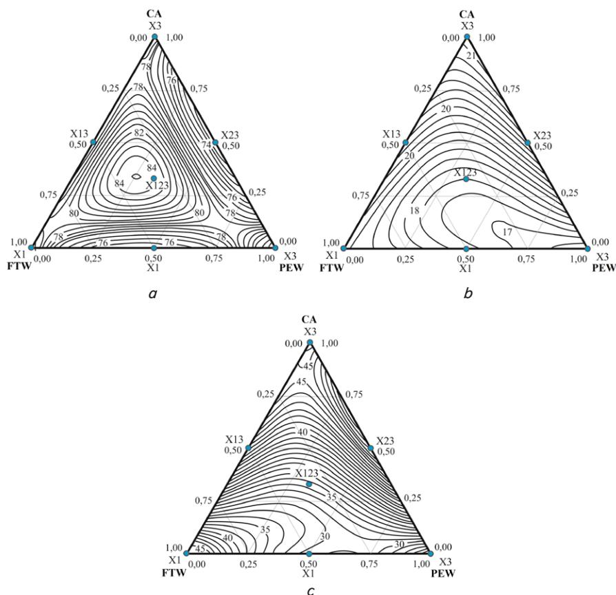
Fig. 1. Dependences of color characteristics of the clinker ceramic materials, obtained under conditions of oxidative annealing, on the composition of masses:  $a$  – lightness  $L^*$ ;  $b$  – coordinate  $a^*$ ;  $c$  – coordinate  $b^*$
