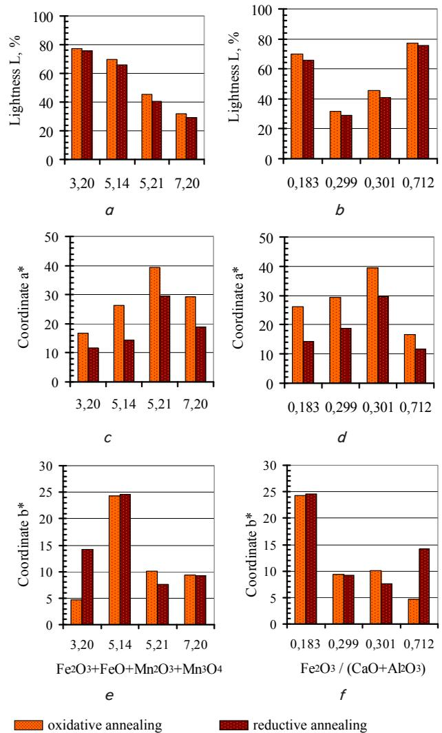
**Fig. 3.** Dependence of color characteristics of ceramic clinker, annealed at a temperature of 1,000 °C on the content of  $\Sigma(\text{Fe}_2\text{O}_3+\text{FeO}+\text{Mn}_2\text{O}_3+\text{Mn}_3\text{O}_4)$  and the ratio of  $\text{Fe}_2\text{O}_3/(\text{Al}_2\text{O}_3+\text{CaO})$ : *a* – lightness  $L^*$ , *b* – coordinate  $a^*$ , *c* – coordinate  $b^*$
