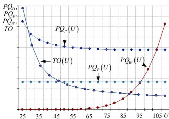
Fig. 4. Dependence of parameters of a process operation on control: control ( $U$ ); power consumption ( $PQ_P$ ); a product of direct effect ( $PQ_D$ ); wear ( $PQ_W$ ); time of the process operation ( $PO$ )
