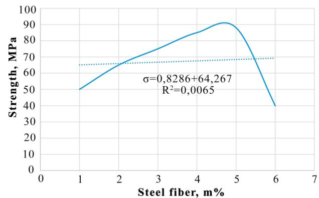
Fig. 6. Plot of fiber-reinforced concrete strength versus steel fiber content
