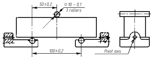
Fig. 4. Layout of the specimen on the bearing elements
