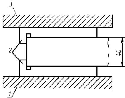
Fig. 5. Specimen position between the pressure plates in the compression test: 1 – lower press plate; 2 – plates; 3 – upper press plate
