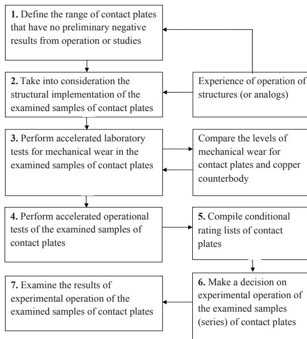
Fig. 3. Procedure for a comparative quality assessment of contact plates
