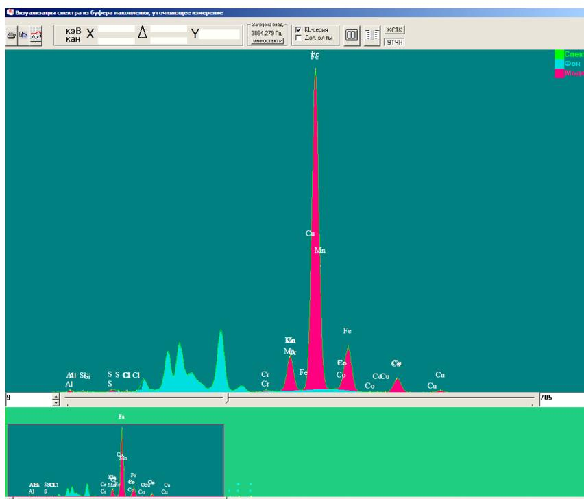
Fig. 2. Results from energy-dispersive analysis of the contact plate BrlG
