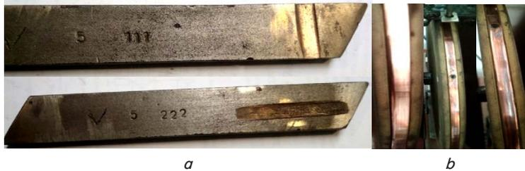
Fig. 5. Results from bench tests of the contact plates BrIG: *a* – contact plates BrIG; *b* – gloss on a contact bus
