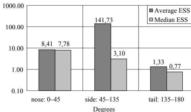
Fig. 5. Average and median values of effective scattering surface for the basic ranges of irradiation azimuths (nose, side, tail)
