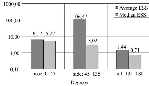
Fig. 10. Average and median values for the “non-coherent” effective scattering surface for the basic ranges of irradiation azimuths (nose, side, tail)
