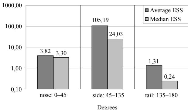
Fig. 15. Average and median values of effective scattering surface for the basic ranges of irradiation azimuths (nose, side, tail)
