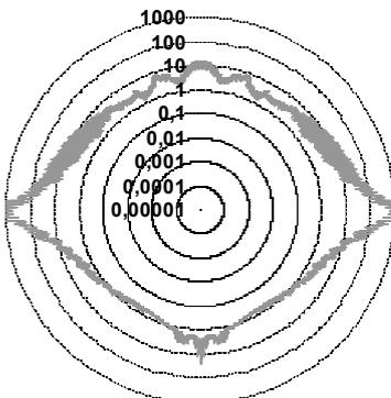
Fig. 9. Pie chart of the “non-coherent” effective scattering surface for the Su-25T anti-tank aircraft model
