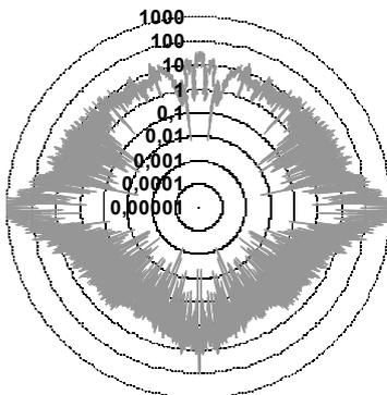
Fig. 8. Pie chart of effective scattering surface for the Su-25T anti-tank aircraft model
