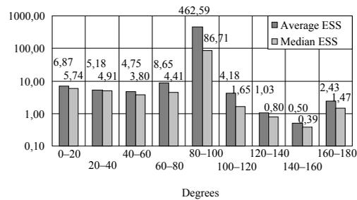
Fig. 11. Average and median value of effective scattering surface for the twenty-degree ranges of irradiation azimuths
