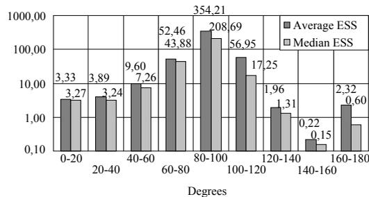
Fig. 16. Average and median values of effective scattering surface for the twenty-degree ranges of irradiation azimuths
