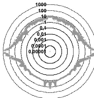
Fig. 4. Pie chart of the "non-coherent" effective scattering surface for the Su-25T anti-tank aircraft model
