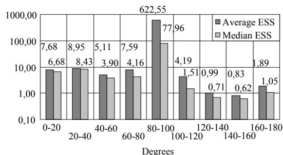
Fig. 6. Average and median values of effective scattering surface for the twenty-degree ranges of irradiation azimuths
