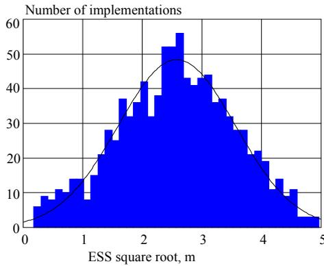
Fig. 7. Histogram of amplitude multiplier (the square root of the values for effective scattering surface) for the reflected signal
