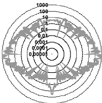
Fig. 13. Pie chart of effective scattering surface for the Su-25T anti-tank aircraft model
