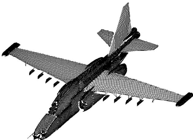
Fig. 2. A model of the Su-25T anti-tank aircraft surface
