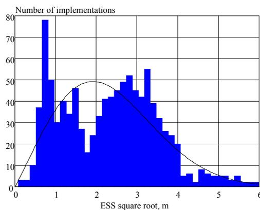
Fig. 12. Histogram of amplitude multiplier (the square root of the values for effective scattering surface) for the reflected signal
