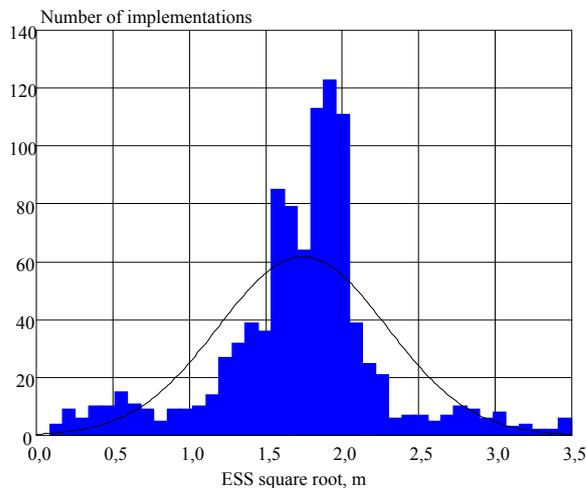
Fig. 17. Histogram of amplitude multiplier (the square root of the values for effective scattering surface) for the reflected signal
