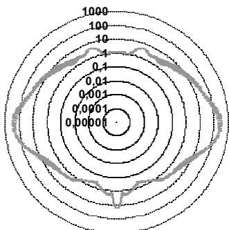
Fig. 14. Pie chart of the “non-coherent” effective scattering surface for the Su-25T anti-tank aircraft model
