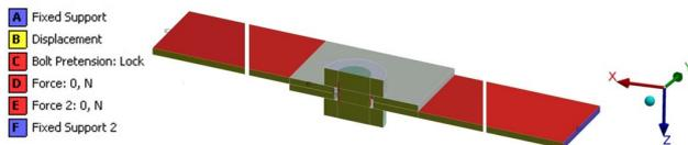
Fig. 8. The test system loading diagram
