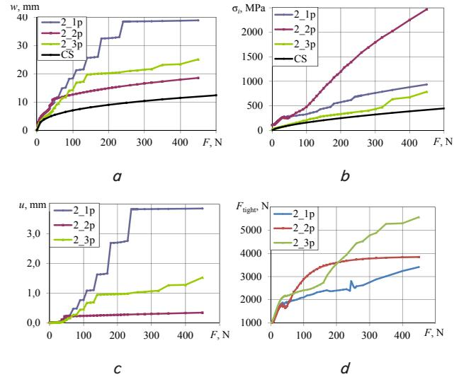
Fig. 14. Results of numerical simulation of the second group at various strip displacements: deflections  $w$ , mm (a); maximum equivalent Mises stresses, MPa (b); displacement of contacting surfaces of strips relative to each other  $u$ , mm (mutual slipping); forces in the bolt under action of loading  $F_{tight}$ , N
