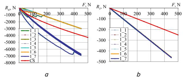
Fig. 10. Reaction in fixtures for all variants of connections depending on external load  $F$ , N: along  $x$  axis  $R_x$ , N (a); along  $z$  axis  $R_z$ , N (b)
