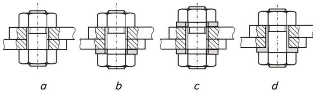
Fig. 4. Group I. Bolted connection arrangement: variable coefficient of friction (bolt-strip, strip-strip, joint washer is absent) (a); variable force of tightening the bolted connection, the washer placed between the bolt head and the strip (b); use of a joint washer at both sides (c); change of the force acting on the upper surface of the strip system (static, cyclic, washer fills the gap) (d)
