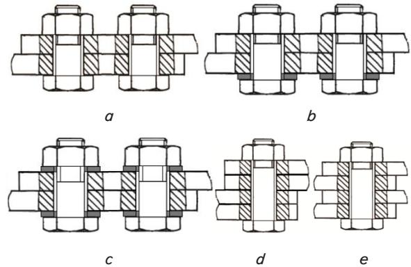
Fig. 6. Group III. Arrangement of bolted connections: two bolted connections without washers (a); two bolted connections with two washers (b); two bolted connections with four washers (c); one bolted connection with two paired strips (d); one bolted connection with two alternately connected strips (e)
