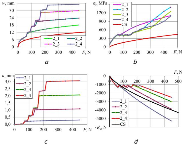
Fig. 13. Results of numerical simulation of the second group for all connection variants: deflection  $w$ , mm (a); maximum equivalent Mises stresses  $\sigma_i$ , MPa (b); displacement of contacting surfaces of the strips relative to each other  $u$ , mm (mutual slipping) (c); reaction in the fixture along  $x$  axis  $R_x$ , N
