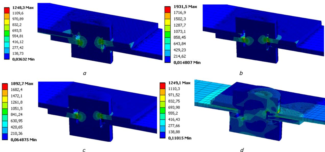
Fig. 11. Distribution of equivalent Mises stresses: variant 1\_1 (a); variant 1\_4 (b); variant 1\_6 (c); variant 1\_7 (d)
