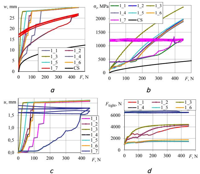
Fig. 9. The results of numerical simulation of the first group for all variants of connections under action of load  $F$ , N: deflection  $w$ , mm (a); maximum equivalent Mises stresses  $\sigma_i$ , MPa (b); displacement of the contact surfaces relative each other  $u$ , mm (mutual slip) (c); force in the bolt  $F_{tight}$ , N (d)
