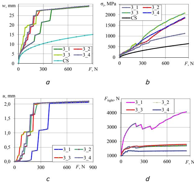
Fig. 15. Results of numerical simulation of the third group for all variants of connections under the action of loading  $F$ , N: deflection  $w$ , mm (a); maximum equivalent Mises stresses  $\sigma_p$ , MPa (b); displacement of contacting surfaces of the strips relative to each other  $u$ , mm (mutual slipping) (c); force in the bolt  $F_{tight}$ , N (d)
