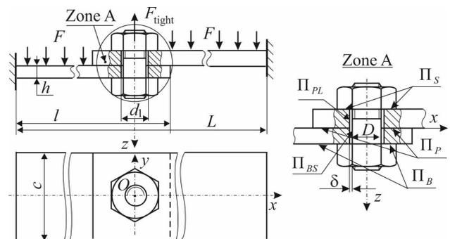
Fig. 3. System of two strips with bolted connection
