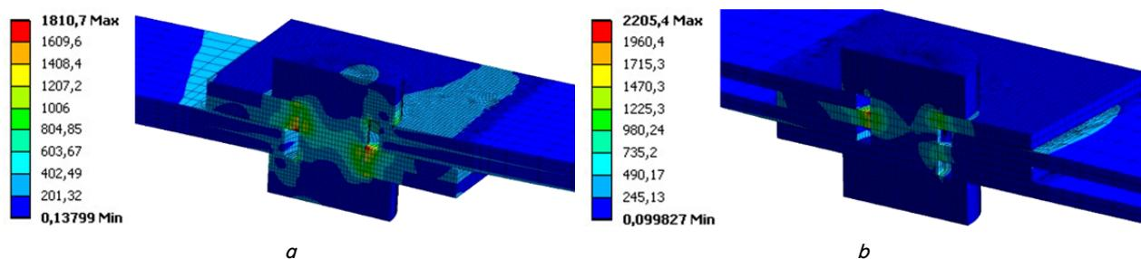
Fig. 18. Distribution of equivalent Mises stresses (Table 3): variant 3\_1p (a); variant 3\_2p (b)
