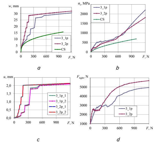
Fig. 17. The results of numerical simulation of the fifth group at different displacement of strips under the influence of load  $F$ , N: deflection  $w$ , mm (a); maximum equivalent Mises stresses  $\sigma_p$ , MPa (b); displacement of contacting surfaces of the strips relative to each other  $u$ , mm (mutual slipping) (c); forces in the bolt  $F_{tight}$ , N (d)
