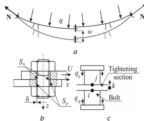
Fig. 1. Diagram of loading of a silo element: diagram of strip connection (a); connection diagram and gaps in the bolted connection (b); model of bolted connection (c)
