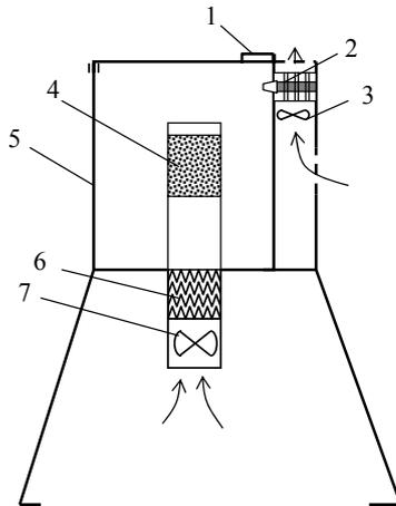
Fig. 1. The scheme of the plant for studying the kinetics of drying grain materials by microwave and convective heating: 1 – door, 2 – magnetron, 3 – magnetron cooling fan, 4 – experimental cell with research material, 5 – working chamber, 6 – electric heater, 7 – fan
