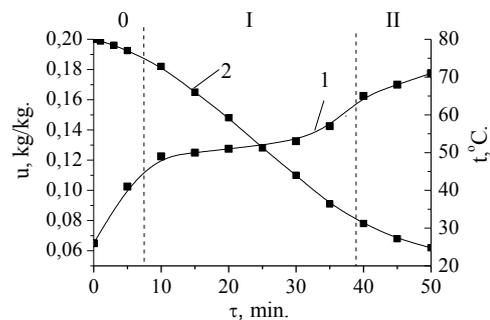
Fig. 2. Change in temperature (1) and moisture content (2) of buckwheat grain when dried in a microwave field.  $P=80 \text{ W}$ ;  $m=0.1 \text{ kg}$ ;  $l=0.016 \text{ m}$ : 0 – heating period, I – period of constant drying rate, II – period of falling drying rate
