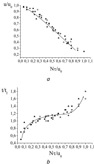
Fig. 4. Generalized drying kinetics curves: a – moisture content curve, b – a temperature curve, ▲ – buckwheat, ■ – barley, ○ – oats, ★ – wheat
