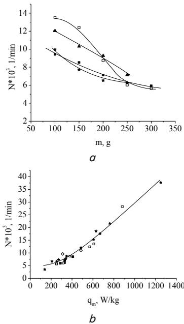
Fig. 3. Dependence of the grain drying rate on variable parameters: a – effect of mass, b – effect of the useful heat flow. ■ – wheat, □ – oats, ▲ – barley, ★ – buckwheat. The output power of the magnetron  $P=180$  W
