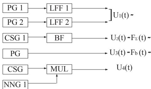
Fig. 5. A scheme of the model of force effects: PG – pulse generators; NNG – normal noise generator; CSG – code-sequence generator; LFF – low frequency filters; BF – bandpass filter; MUL – multiplier
