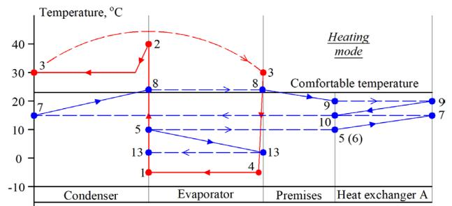
Fig. 6. Energy flows in the system “premises – refrigerating machine” in the heating mode
