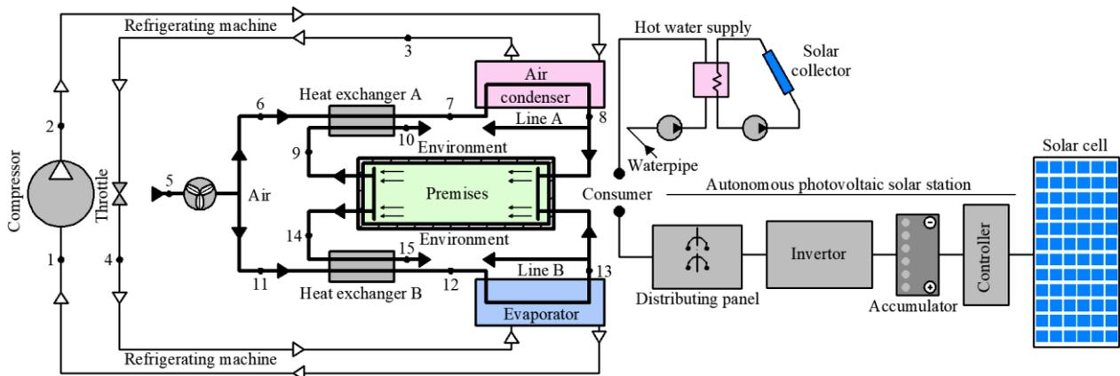
Fig. 4. Generalized technological scheme of a small trigeneration system
