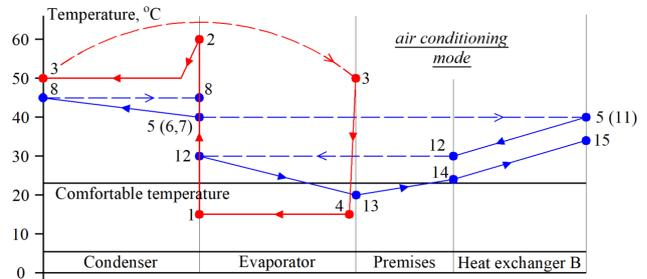
Fig. 5. Energy flows in the system “premises – refrigerating machine” in the air conditioning mode
