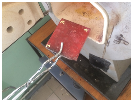
Fig. 2. Physical appearance of labradorite sample when heated to 800 °C
