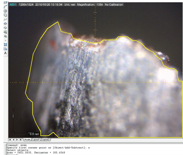
Fig. 7. Surface area of tool wear model 7
