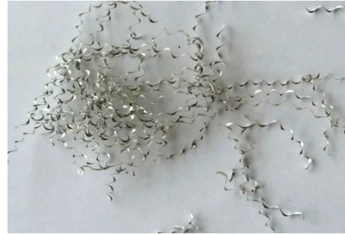
Fig. 10. Continuous chip visualization on model 7 with a 1.2 mm nose radius
