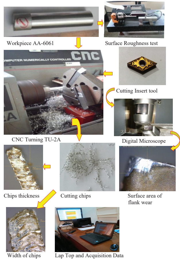
Fig. 3. Experimental design (Department of Mechanical Engineering CNC, Industrial Metrology and Metallography Laboratory, University of Merdeka Malang)
