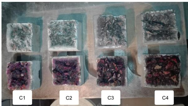
Fig. 4. Carbonization of alkaline concretes that included water treatment waste
