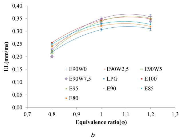
Fig. 6. Laminar burning velocity ( $U_L$ ):  $a$  – various fuel compositions;  $b$  – Hydrus E90
