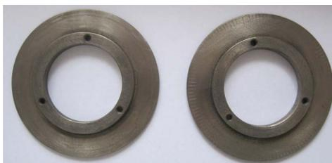
Fig. 17. Knitting equipment with ZrN coated wheels
