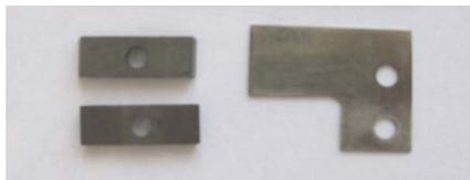
Fig. 15. Knitting equipment knives with ZrN coating
