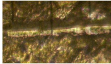
Fig. 11. Results of sclerometric studies of coatings on VSt3sp steel with a load of 15 g on the indenter after 80 min implantation of Cr and N ions  $\times 800$
