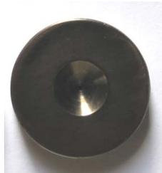
Fig. 14. Spinneret of 40X steel with CrN coating
