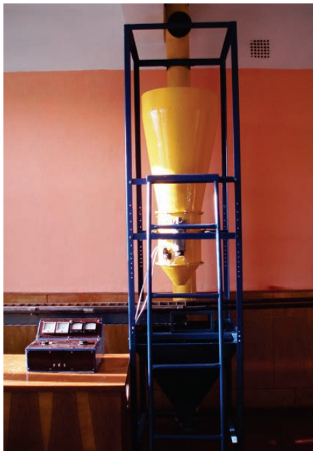
Fig. 5. Laboratory setup for studying the process of feed dosing
