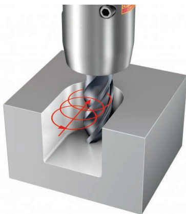
Fig. 4. Schematic of trochoidal milling of a wide groove
