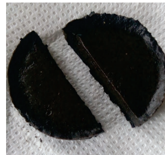
Fig. 3. Sediment after deliquescence in a laboratory chamber-membrane filter press with addition of fly ash
