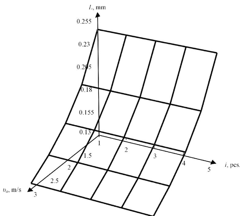
Fig. 3. Dependence of length of the bristle rod on the assembly's translational velocity  $v_a$  and the number of bristles in a bundle  $i$
