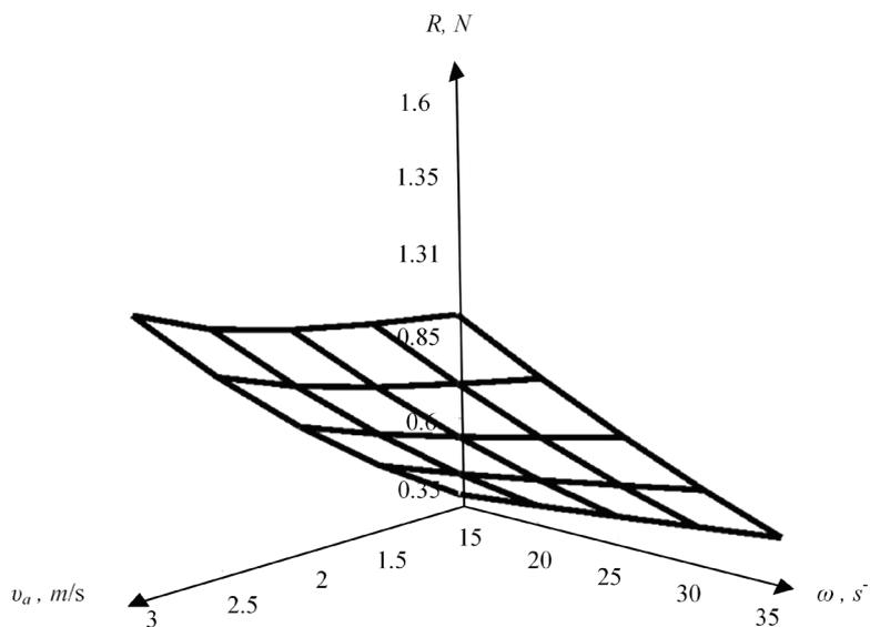
Fig. 2. Dependence of the resultant resistance force to the displacement of a bristle rod on the assembly's translational speed  $v_a$  and the brush angular velocity  $\omega$
