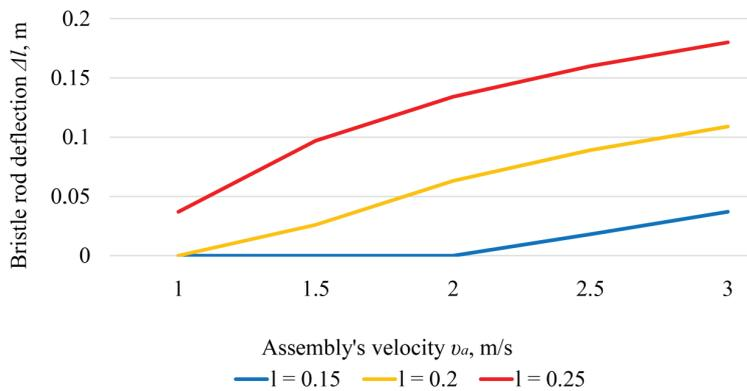
Fig. 4. Dependence of deflection  $\Delta/l$  of bristle rods on their length  $l$  and the assembly's working velocity  $v_a$
