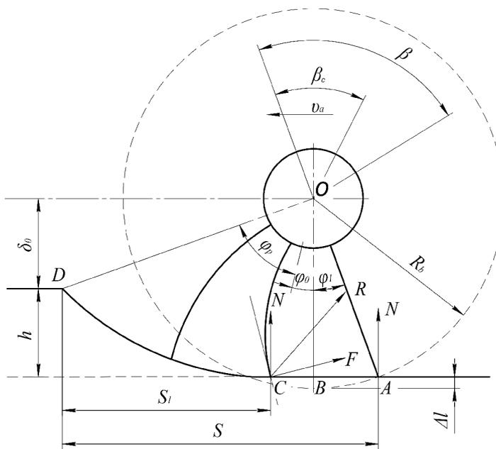
Fig. 1. Diagram of brush operation
