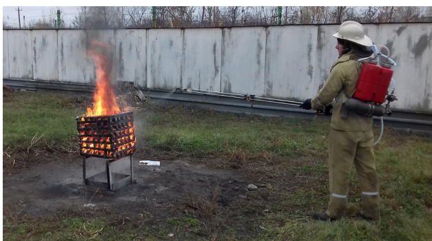
Fig. 4. Extinguishing the simulation fire 1A by the installation with the extended barrel of the cranked type for extinguishing by gel-forming compositions
