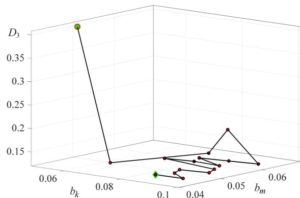
Fig. 5. Path to solve the optimization problem for the parameters of an electromechanical shock absorber using the method of genetic algorithm in coordinates  $b_k$ ,  $b_m$ ,  $D_3$
