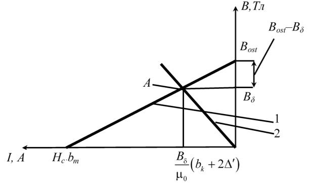
Fig. 2. Determining the induction of a magnetic field in the air gap: 1 – magnetic characteristic of permanent magnet; 2 – magnetic characteristic of air gap
