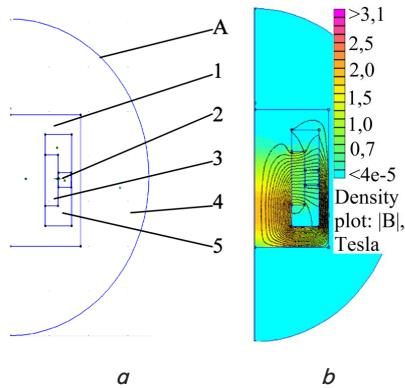
Fig. 3. Calculation of the magnetic field of a shock absorber using the method of finite elements at working travel  $\Delta=40$  mm: *a* – estimated area; *b* – results from calculating a magnetic field
