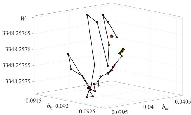
Fig. 8. Path to solve the optimization problem for the parameters of an electromechanical shock absorber using the Nelder-Mead method in coordinates  $b_k, b_m, W$
