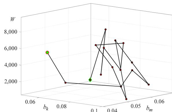
Fig. 6. Path to solve the optimization problem for the parameters of an electromechanical shock absorber using the method of genetic algorithm in coordinates  $b_k$ ,  $b_m$ ,  $W$
