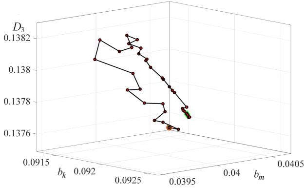
Fig. 7. Path to solve the optimization problem for the parameters of an electromechanical shock absorber using the Nelder-Mead method in coordinates  $b_k, b_m, D_3^\circ$
