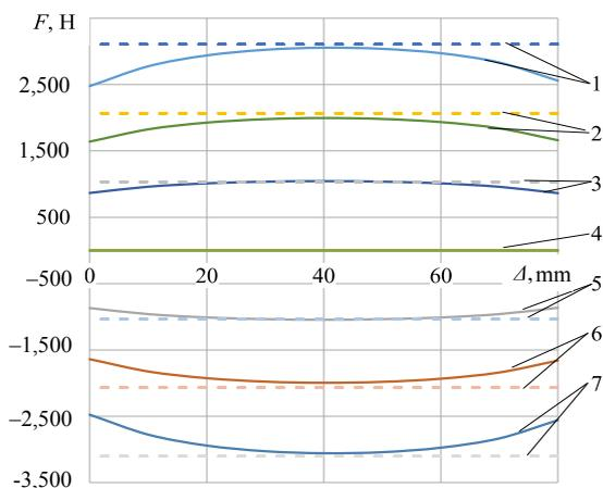
Fig. 4. Mechanical characteristics of shock absorber at the winding m.m.f.: 1 – 7,780 A; 2 – 5,120 A; 3 – 2,590 A; 4 – 0 A; 5 – –2,580 A; 6 – –5,120; 7 – –7,780 A, dotted line indicates values derived in line with (6)
