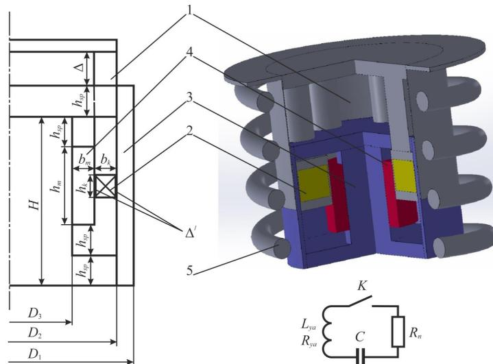
Fig. 1. Mechanical shock absorber of direct current: 1 – armature; 2 – armature winding; 3 – bed; 4 – permanent magnet; 5 – spring
