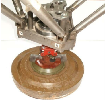
Fig. 11. The gripping device used to experimentally determine the momenta of screwing and loosening the fuse
