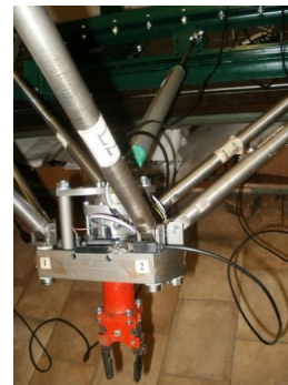
Fig. 9. Installing a special grip on a movable platform of the manipulator
