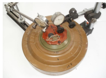
Fig. 14. Installing indicators on the ATM mockup for measuring the fuse transverse-angular displacements
