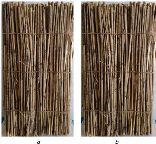
Fig. 1. Model samples of heat-insulating mats made from reed: a – untreated; b – treated with the modified roofing impregnating solution «Skela-i»
