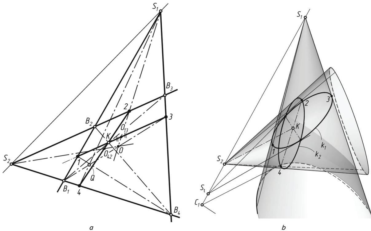
Fig. 3. Full-scale image of the plane of centers and modeling cross-sections of inscribed surface: *a* – image of the full-scale of the plane of centers; *b* – contact line of inscribed surface
