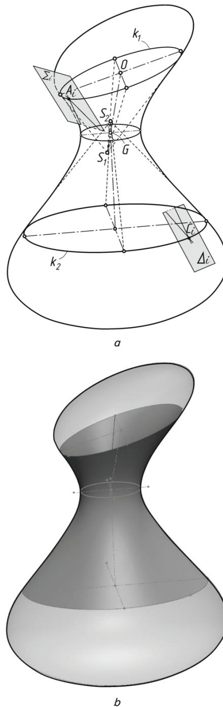
Fig. 7. Modeling the surfaces from three conjugate quadrics: *a* – geometric scheme; *b* – appearance
