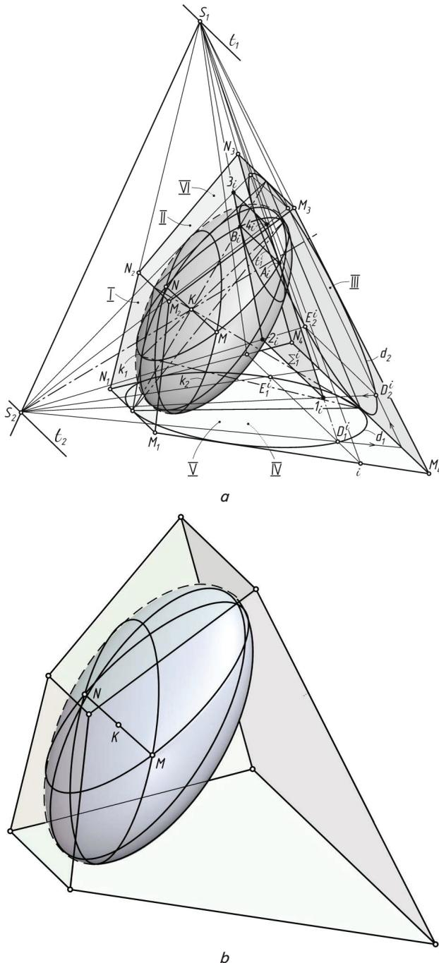
Fig. 5. A hexagon, which limits the quadric surface, assigned by two tangent cones:  $a$  – geometric scheme of construction of quadric;  $b$  – images of the quadric that is tangent to the hexagon faces
