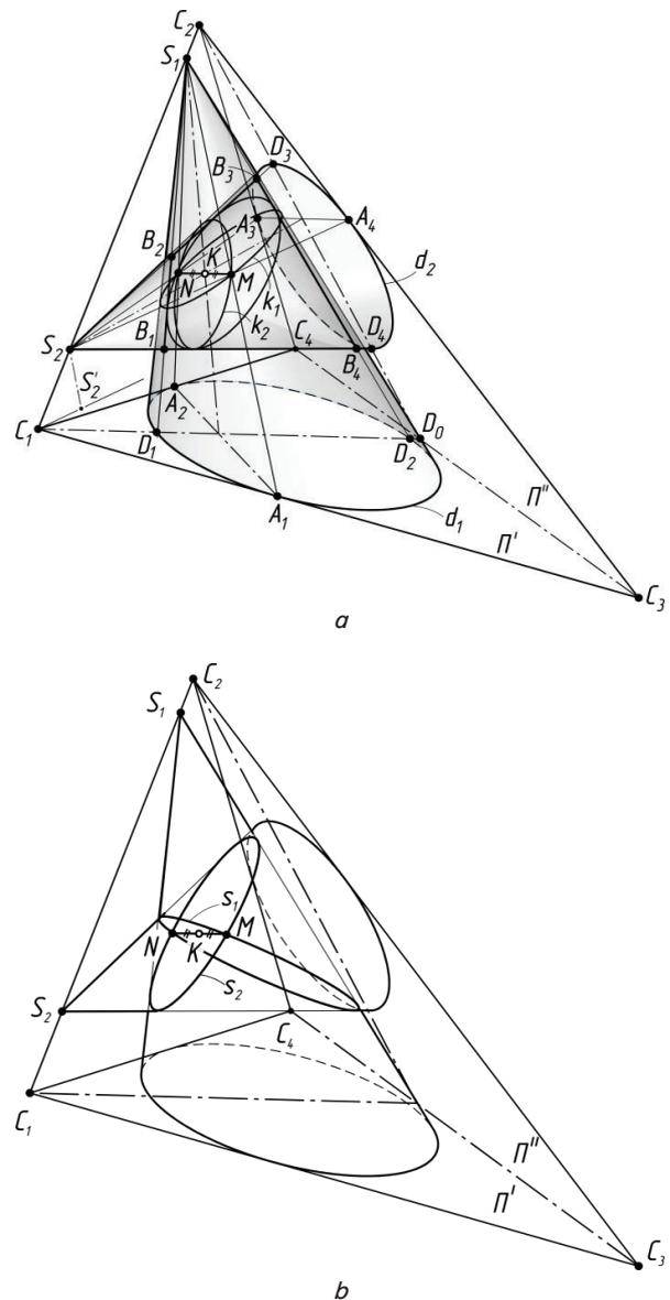
Fig. 2. The variant of construction of the geometric structure:  $a$  – geometric scheme;  $b$  – cross-section of quadric cones by flat curves
