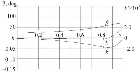
Fig. 8. Distribution of curvature  $k$ , curvature derivative  $k'$  and angle  $\beta$  depending on the relative length of curve for the pressure side of the nozzle blade profile
