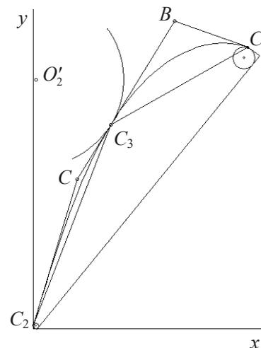
Fig. 3. Result of modeling the suction side of profile
