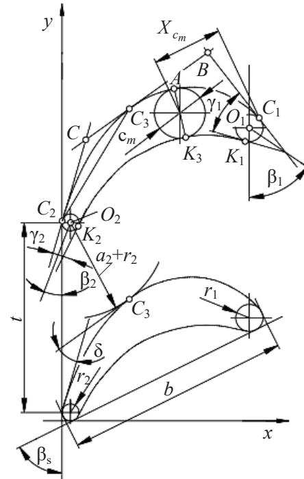
Fig. 1. Profiles of turbine blades and their geometric parameters
