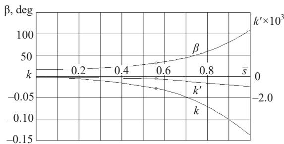
Fig. 4. Distribution of curvature  $k$ , its derivative  $k'$  and angle  $\beta$  depending on relative curve length for the suction side of the nozzle blade profile
