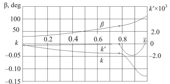
Fig. 11. Distribution of curvature  $k$ , curvature derivative  $k'$  and angle  $\beta$  depending on the relative length of the curve for the pressure side of the rotor blade profile
