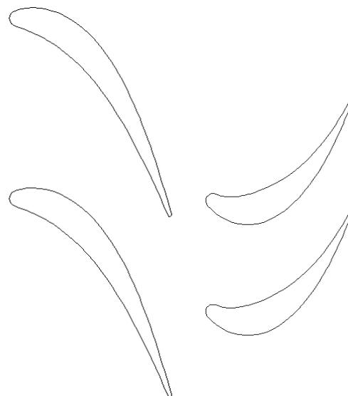
Fig. 12. Profiles of the nozzle and working blades of the turbine stage
