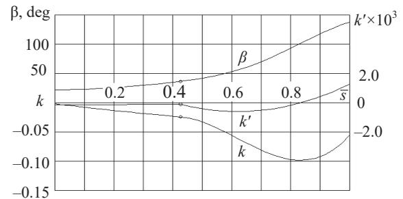
Fig. 10. Distribution of curvature  $k$ , curvature derivative  $k'$  and angle  $\beta$  depending on the relative length of the curve for the suction side of the rotor blade profile
