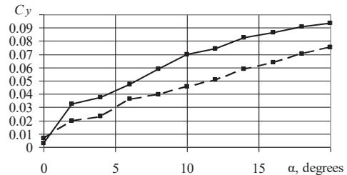
Fig. 5. Dependence of lift force coefficient  $C_y$  on angle of attack  $\alpha$ : - - - - - TJDE nacelle; — — — — — stepped nacelle for engine with TFU
