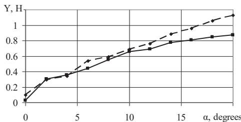
Fig. 3. Dependence of lift force  $Y$  on angle of attack  $\alpha$ : - - - - - TJDE nacelle; — — — — — stepped nacelle for engine with TFU
