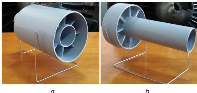
Fig. 1. Nacelle models for conducting experimental study: *a* – model of TJDE nacelle; *b* – model of stepped nacelle for GTE with TFU
