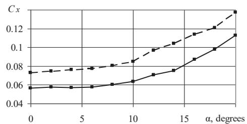
Fig. 6. Dependence of aerodynamic drag coefficient  $C_x$  on angle of attack  $\alpha$ : - - - - - TJDE nacelle; — — — — — stepped nacelle for engine with TFU
