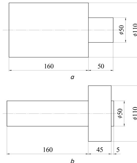
Fig. 2. Diagrams and basic geometrical parameters of nacelles for powerplants: *a* – TJDE nacelle; *b* – stepped nacelle for GTE with TFU
