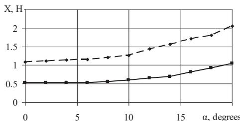
Fig. 4. Dependence of aerodynamic drag force  $X$  on angle of attack  $\alpha$ : - - - - - TJDE nacelle; — — — — — stepped nacelle for engine with TFU
