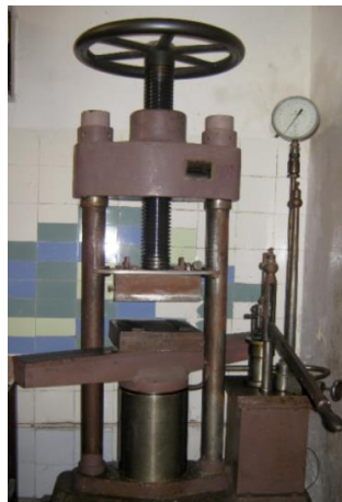
Fig. 1. Hydraulic press used to form fuel briquettes
