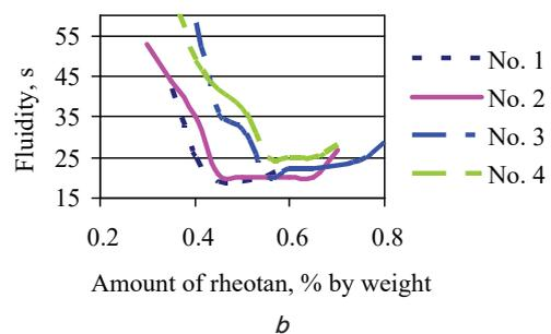
Fig. 3. Indicators of fluidity of the studied slips at dilution: *a* – with liquid glass; *b* – rheotan
