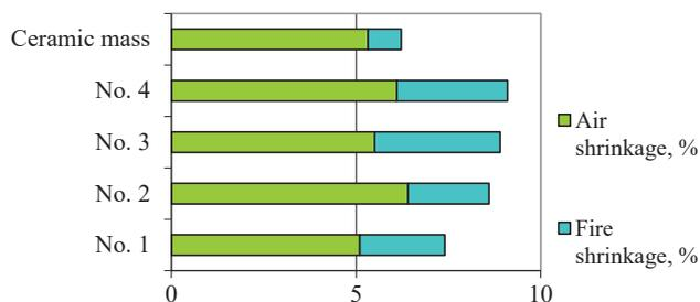
Fig. 5. Indicators of shrinkage of ceramic mass and studied engobes
