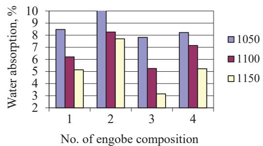
Fig. 4. Indicators of water absorption for engobe samples after annealing at different temperatures
