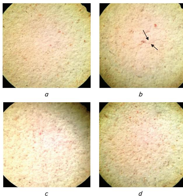
Fig. 6. External view of engobe surface of the samples after annealing at 1,100 °C, magnification  $\times 32$ : a – No. 1, b – No. 2, c – No. 3, d – No. 4
