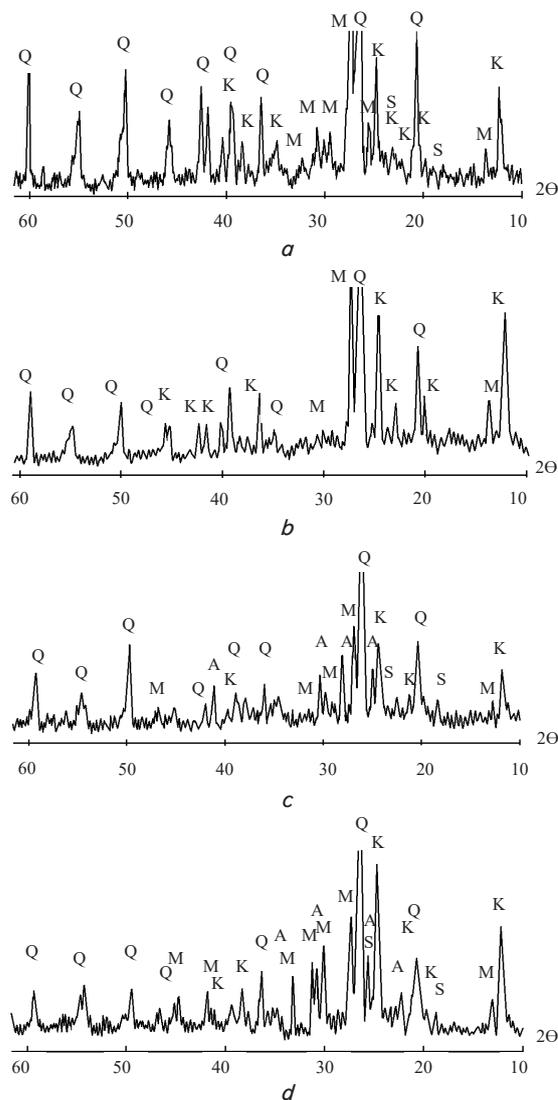
Fig. 1. X-ray phase analysis of samples of alkaline kaolins from: *a* – Katerynivsky; *b* – Maidan-Vilsky; *c* – Yosypivsky; *d* – Nemylniansky deposits; K – kaolinite; Q –  $\beta$ -quartz; M – microcline; A – albite; S – mica
