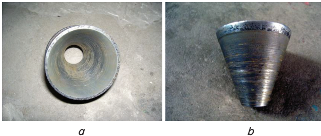
Fig. 12. Signs of abrasive-corrosion wear in the components from a friction pair in the slide frame of a mortar mixer: a – insert; b – wrist pin
