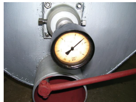
Fig. 9. Determining the axial load on a frame by the device
