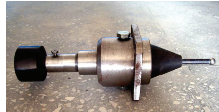
Fig. 8. Image of the device for determining the axial load
