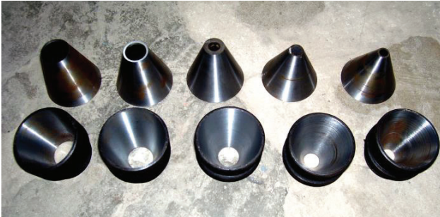
Fig. 10. Examined samples of the wrist pin in a slide frame at angle \alpha at the apex: 30°, 35°, 40°, 45°, 50° (from left to right)
