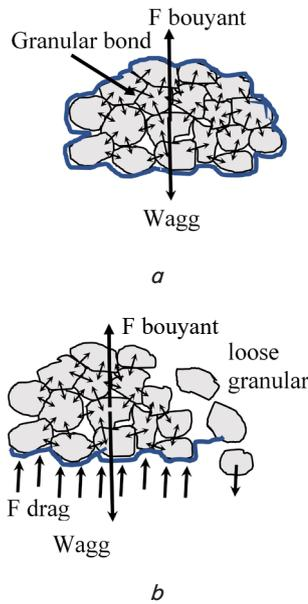
Fig. 4. Forces are acting on granular agglomerate: *a* – granular agglomerate; *b* – drag force breaking the bonds
