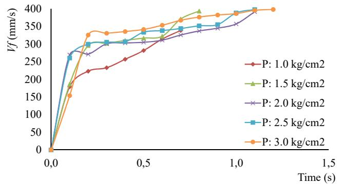
Fig. 12. Fluidized movement ( $V_f$ ) at the diameter of granular 290 μm
