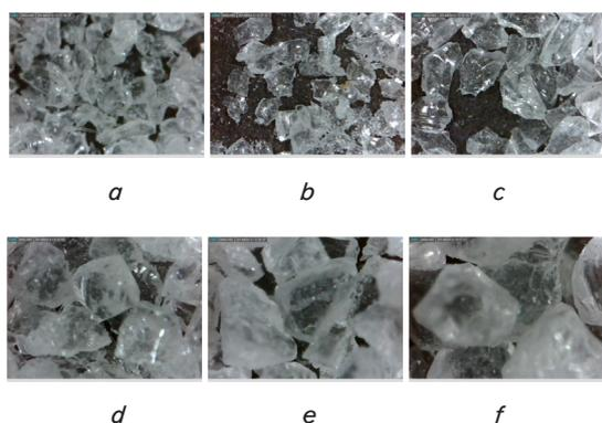
Fig. 2. Granular materials for the experiment: a – 80 μm; b – 100 μm; c – 140 μm; d – 230 μm; e – 290 μm; f – 340 μm
