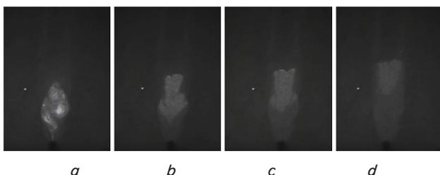
Fig. 6. Movement of 100  $\mu\text{m}$  granular by impinging for 0.1 s with a pressure of 2.0  $\text{kg}/\text{cm}^2$  into the granular bed: *a* – 0.5 s; *b* – 1.0 s; *c* – 7.5 s; *d* – 12 s
