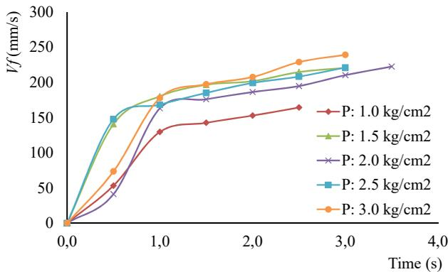
Fig. 11. Fluidized movement ( $V_f$ ) at the diameter of granular 230 μm
