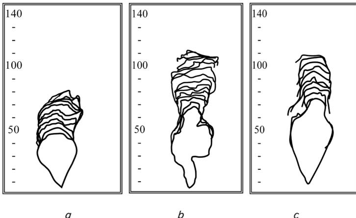
Fig. 13. Patterns of granular motion by impinging for 0.1 s with a pressure of 2.0 kg/cm<sup>2</sup>: a – 80 μm; b – 100 μm; c – 140 μm
