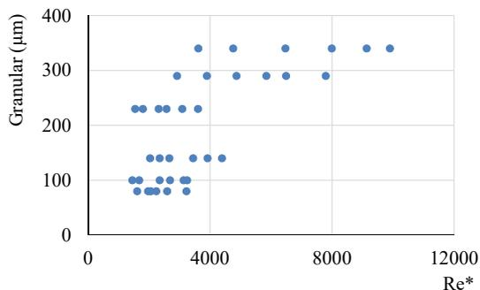
Fig. 15. Reynolds number on differences in granular diameter at impinging 0.1 s
