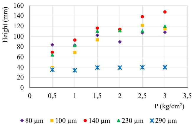
Fig. 14. Height of fluidization at post-impinging vs impinging pressure
