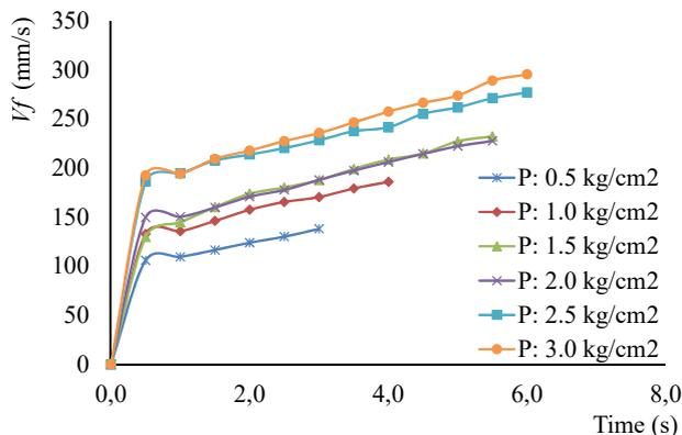
Fig. 9. Fluidized movement ( $V_f$ ) at the diameter of granular 140  $\mu\text{m}$
