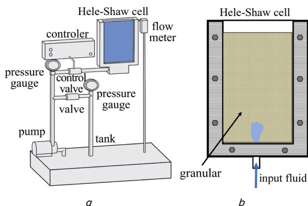
Fig. 1. Equipment for observation of fluidization: a – arrangement of equipment; b – Hele-Shaw cell
