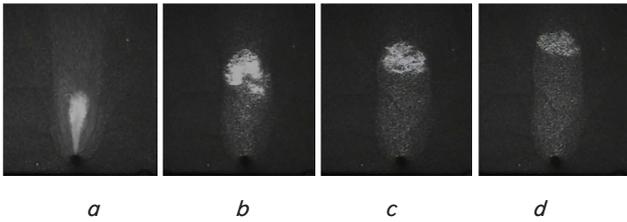
Fig. 10. Visualization of motion of 230 μm granular by impinging 0.1 s with a pressure of 2.0 kg/cm<sup>2</sup> into the granular bed: a – 0.3 s; b – 0.9 s; c – 1.5 s; d – 2.5 s
