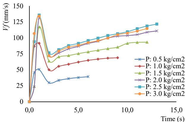
Fig. 7. Fluidized movement ( $V_f$ ) at the diameter of granular 100  $\mu\text{m}$
