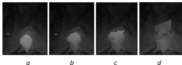
Fig. 3. Movement of 80 μm granular by impinging for 0.1 s at a pressure of 2.0 kg/cm<sup>2</sup> into the granular bed: a – 0.5 s; b – 10 s; c – 20 s; d – 23 s
