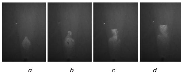
Fig. 8. Movement of 140  $\mu\text{m}$  granular by impinging for 0.1 s with a pressure of 2.0  $\text{kg}/\text{cm}^2$  into the granular bed: *a* – 1.0 s; *b* – 1.5 s; *c* – 2.0 s; *d* – 4.0 s
