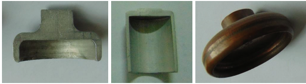
Fig. 6. Hollow components obtained by the radial-direct extrusion with expansion
