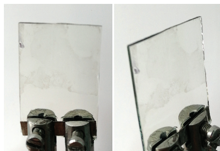
Fig. 4. Results for the film, aged for 8 hours at 80 °C in 0.1 M KOH (KOH sample): a – CV; b – coloration-bleaching curve; c – photographs of the electrode in the colored state after cycling
