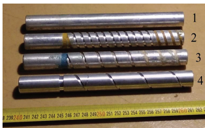
Fig. 2. Investigated heat transfer surfaces: 1 – cylinder with a smooth surface; cylinders with spiral grooves; 2 – S=10 mm; 3 – S=20 mm; 4 – S=40 mm
