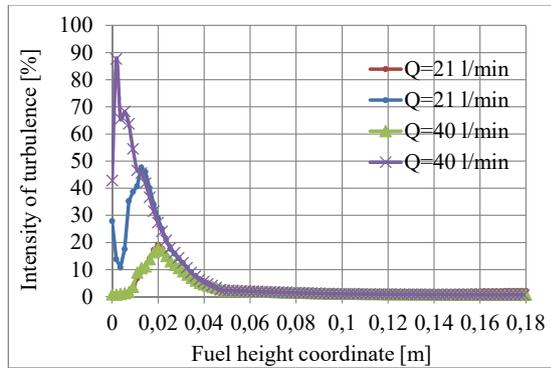
Fig. 18. Graphic dependence of the intensity of turbulence of foam jets of different productivity on the fuel height coordinate
