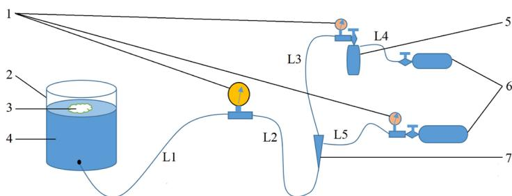
Fig. 8. A block diagram of the experimental unit: 1 – manometers; 2 – a metal tank; 3 – foam; 4 – motor fuel; 5 – a tank with a foam concentrate solution (fire extinguisher); 6 – a cylinder with compressed air or inert gas; 7 – an injector (glass)
