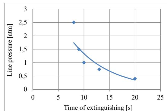
Fig. 20. Graphic dependence of the extinguishing time on the pressure in the line
