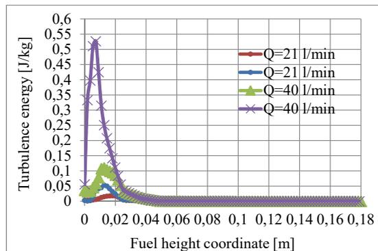
Fig. 19. Graphic dependence of turbulence energy of foam jets of different productivity on the tank height coordinate
