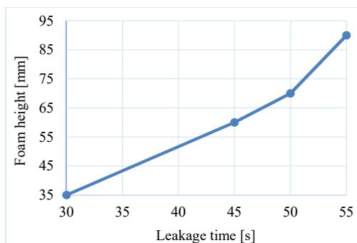
Fig. 9. Dependence of the foam height throughout the surface of the fuel on the leakage time
