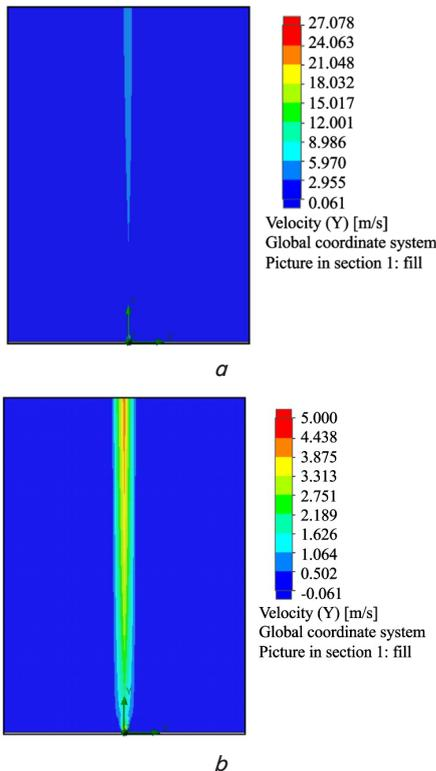
Fig. 3. A chromatogram of the vertical medium velocity: *a* – unfiltered; *b* – filter 5 m/s
