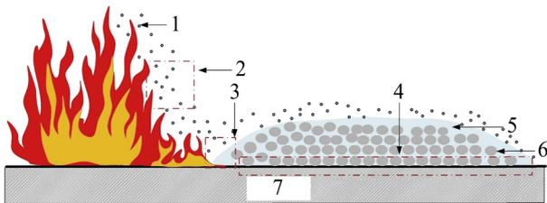
Fig. 1. A schematic diagram of the fire extinguishing mechanism by AFFF during the combustion of diesel fuel: 1 – water vapour; 2 – a rarefaction effect; 3 – cooling; 4 – an insulating effect; 5 – an aqueous film; 6 – a foam layer; 7 – diesel fuel
