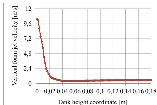
Fig. 13. Graphic dependence of the vertical foam jet velocity on the fuel height coordinate
