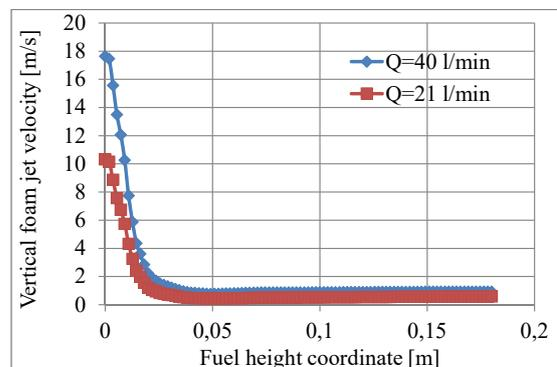
Fig. 17. Dependence of the vertical velocity of foam jets of different productivity on the fuel height coordinate
