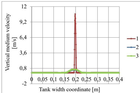
Fig. 14. Graphic dependence of the vertical velocity of the tank on its width at different levels of fuel height: 1 – the bottom of the tank; 2 – the middle of the fuel level; 3 – the top of the fuel
