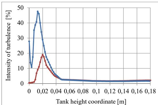
Fig. 15. Graphic dependence of turbulence intensity on the fuel height coordinate: the red line – in the centre of the jet; the blue line – 6 cm shifted to the left to the maximum value
