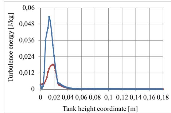
Fig. 16. Graphic dependence of turbulence energy on the fuel height coordinate
