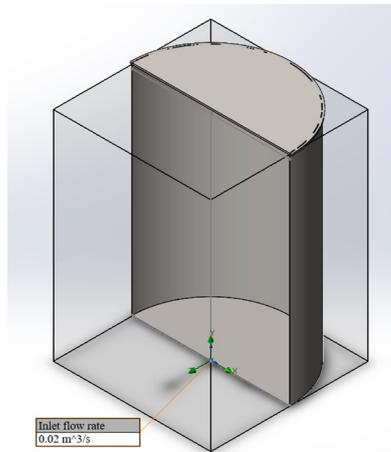
Fig. 2. A tank model with a vertical foam injection
