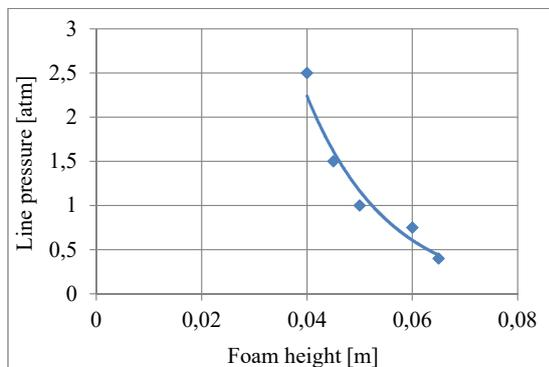
Fig. 21. Graphic dependence of the height of the foam layer on the pressure in the line
