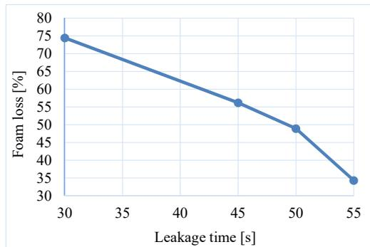
Fig. 10. Dependence of the foam loss throughout the fuel surface on the leakage time
