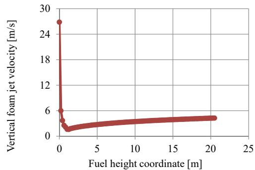
Fig. 4. Dependence of the vertical velocity of the foam jet on the tank height coordinate
