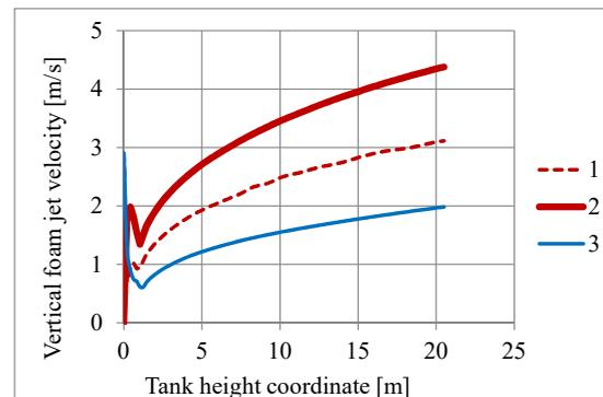
Fig. 7. Dependence of the vertical velocity of the combined foam jet on the fuel height coordinate (line 1 – in the centre of one of the ten foam jets; line 2 – in the centre of a jet comprised of the ten foam jets; and line 3 – in the centre of a separate single foam jet with similar output parameters)
