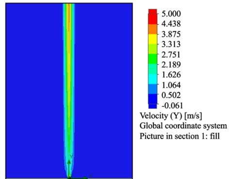
Fig. 6. A chromatogram of the vertical foam jet velocity
