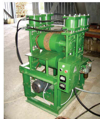
Fig. 1. Experimental installation to flatten branches [13]
