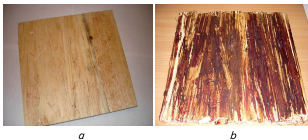
Fig. 3. The panels made using the following binder: a – urea formaldehyde resin, b – phenol-formaldehyde resin
