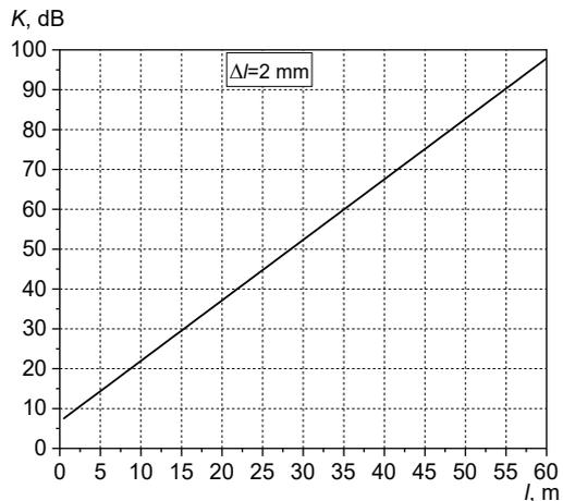
Fig. 5. Dependence of the transmission coefficient of a non-uniform line on the line length at  $\Delta=2$  mm
