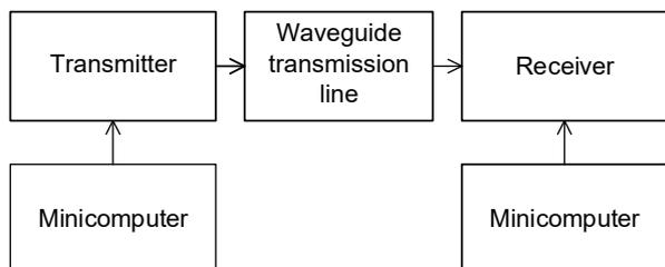
Fig. 1. Block diagram of waveguide transmission of data on the spatial position of the piercing head
