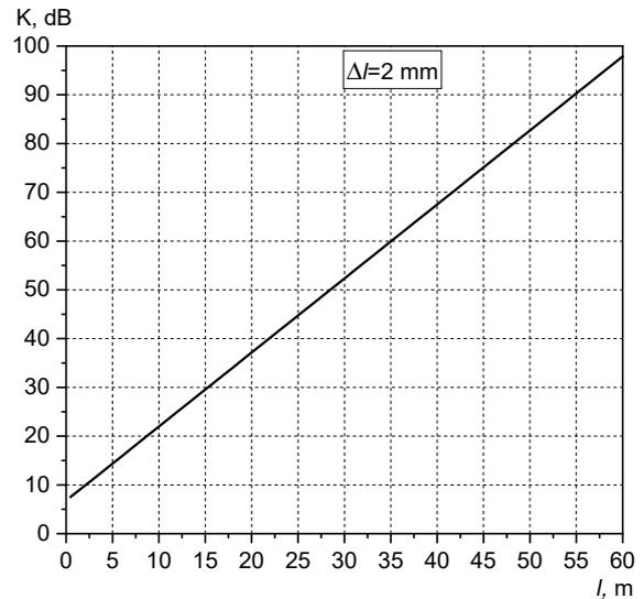
Fig. 7. Increase in the transmission coefficient of a non-uniform line in comparison with a uniform line depending on the line length
