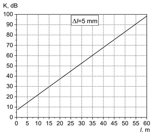
Fig. 6. Dependence of the transmission coefficient of a non-uniform line on the line length at  $\Delta=5$  mm
