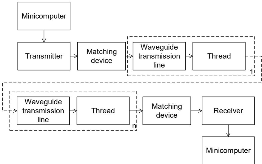
Fig. 2. Measuring channel of determining the spatial position of the piercing head
