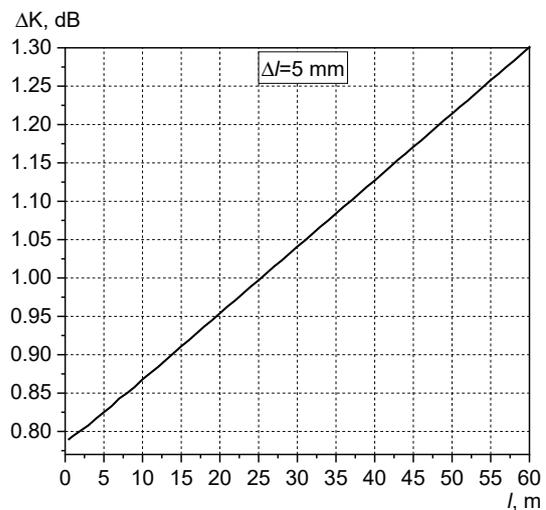
Fig. 8. Increase in the transmission coefficient of a non-uniform line in comparison with a uniform line depending on its length
