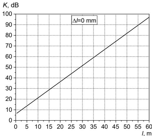
Fig. 4. Dependence of the transmission coefficient of a uniform line on the line length
