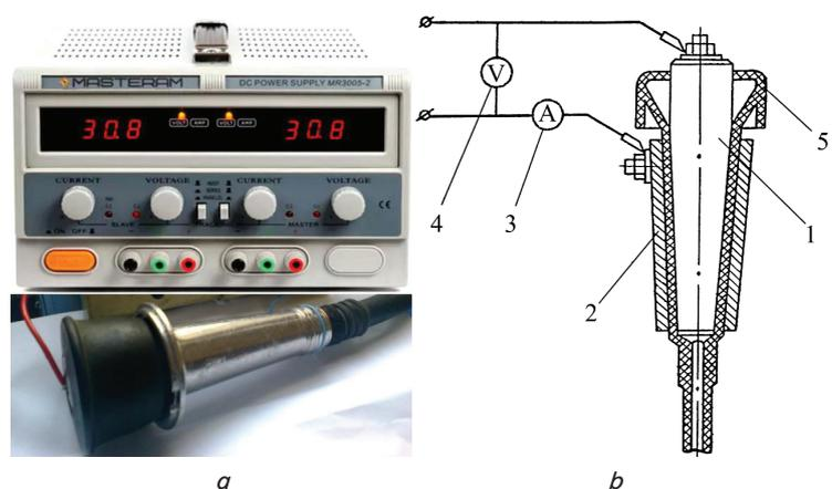
Fig. 1. Device for finding defects in the milking rubber of milking cups using an electric current: *a* – physical appearance of the device with the adjustable power supply unit Masteram MR3005-2; *b* – the scheme of the device: 1 – conic core; 2 – cartridge; 3 – electric current meter; 4 – current voltage meter; 5 – the examined milking rubber [26]
