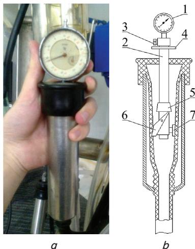
Fig. 3. Device for determining the tension of milking rubber in milking cups: *a* – physical appearance; *b* – device diagram: 1 – counting unit; 2 – body; 3 – fixing screw; 4 – stop; 5 – movable bushing; 6 – rotary lever; 7 – stationary insert
