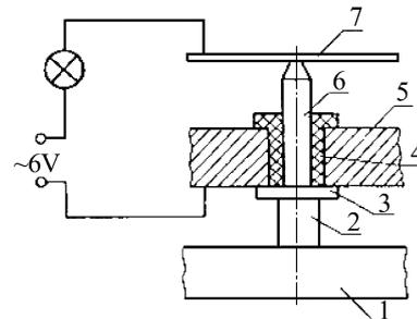
Fig. 2. Electro-mechanical diagram for determining an aging coefficient based on compression stress: 1 – lower plate; 2 – a sample of milking rubber; 3 – flange; 4 – guide bushing; 5 – upper plate; 6 – rod; 7 – spring
