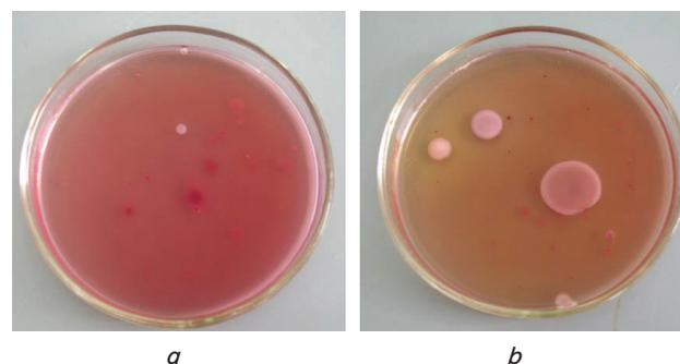
Fig. 7. Bacterial insemination of milking rubber: a – after 3 months of operation; b – after 6 months of operation
