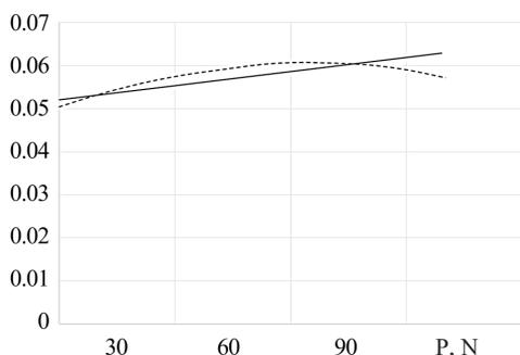
Fig. 6. Dependence of the duration of the deformation loss by the milking rubber shell on the value of its tension in the sleeve of the milking cup: — — linear dependence  $y=0.001x+0.053$  ( $R^2=0.6$ ); - - - - polynomial dependence  $y=-0.0003x^2+0.0035x+0.0505$  ( $R^2=0.9333$ )
