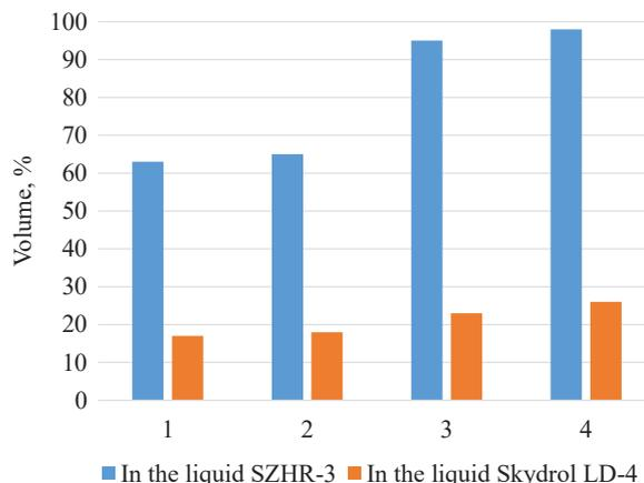
Fig. 5. Change in the volume of milking rubber in the environment of liquids at  $t=150\text{ }^{\circ}\text{C}$  for 72 hours: 1 – rubber Bou Matic (analog to DD.00.041A) from the material of food silicone; 2 – rubber De Laval (analog to DD.00.041A) from the material of rubber compounds; 3 – rubber DD 00.041A from the material of rubber compounds manufactured by AO «Bratslav»; 4 – rubber DD 00.041A from the material of rubber compounds manufactured by AT «Agrotechimport»
