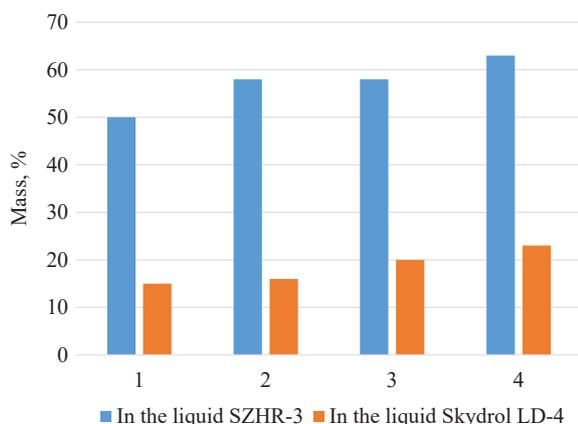
Fig. 4. Change in the mass of milking rubber in the environment of liquids at  $t=150\text{ }^{\circ}\text{C}$  for 72 hours: 1 – rubber Bou Matic (analog to DD.00.041A) from the material of food silicone; 2 – rubber De Laval (analog to DD.00.041A) from the material of rubber compounds; 3 – rubber DD 00.041A from the material of rubber compounds manufactured by AO «Bratslav»; 4 – rubber DD 00.041A from the material of rubber compounds manufactured by AT «Agrotechimport»
