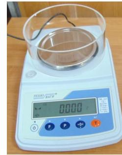
Fig. 3. Laboratory scales TVE-0.21-0.001
